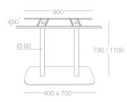
Model Base FEET TOP APPLICABLE TABLE TOP Kg. SUPPORT MAXIMUM RECOMENDED SIZE 400 x 750 table base 400 x 750 H. 730 450 x 900 800 x 1400 Kg. 26,5 Ø 60 400 x 750 bar table base 400 x 750 H. 1100 450 x 900 700 x 1100 Kg. 28 Ø 60
